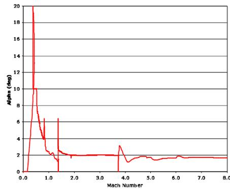
**Figure 10. Alpha vs. Flight Mach Number**
