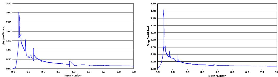
**Figure 11. Lift and Drag Coefficients vs. Flight Mach Number**
